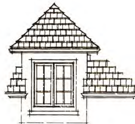
HIPPED THROUGH THE CORNICE
